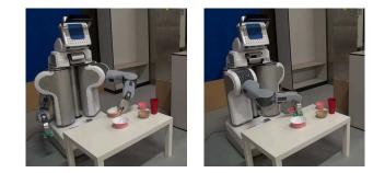
Fig. 1. This figure shows the PR2 robot during the execution of a tidy up task. The robot picks up a bowl to wipe the spot where it was placed.
