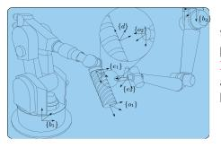
In order to find the joint angles of the second robot the robot programmer has to find **PoseCoord** ( $\{e_2\}|\mathcal{E}_2, \{b_2\}|\mathcal{B}_2, [b_2]$ ), and subsequently use the inverse kinematics of the second robot.
