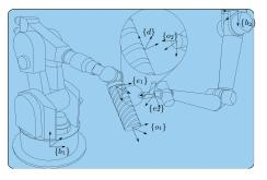
**Goal =** determine the joint angles of the second robot holding the spray gun such that a predefined pose between the spray gun and cylindrical object is obtained
