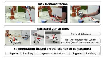
Fig. 1. Encoding a demonstrated task based on extracted constraints and segmenting it into reaching and manipulation parts when constraints change.
